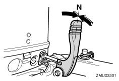
Place the tilt lock lever in the release/up position.
